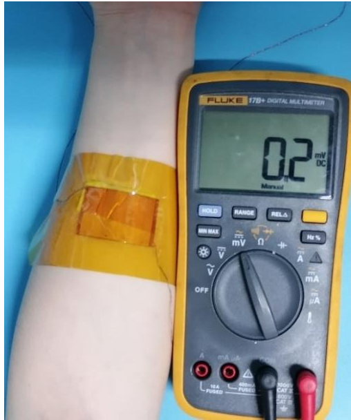
Figure S15. The photo of output voltage of the TEG fixed on the wrist at room temperature.
